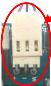
Do ensure that the pins connected to encoder are correct. (+) for VCC, (-) for GND and (s) for signal.
