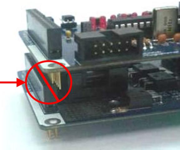
**Cautions:** Please ensure that all card pins are not shifted when stacking. IFC system will NOT function if the pins are shifted.
