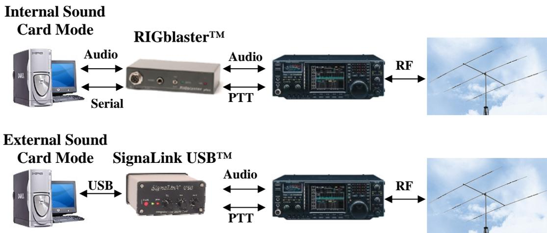
Figure 1 shows a typical sound card interface options for an amateur radio transceiver. All audio cables are shielded. Some sound card interfaces have USB rather than RS-232 serial port capability. Some Sound Card Interfaces connect to the microphone input (MIC & PTT) and speaker output, while others connect entirely to an accessory
