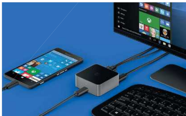
Using a $99 DisplayDock accessory, you can attach certain Windows 10 phones to a monitor and use them like a PC.
