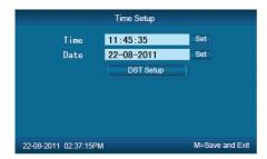
【Time/ Date】 Set the device time and date .The device time date and time should be correct in order to guarantee the attendance time is correct.
