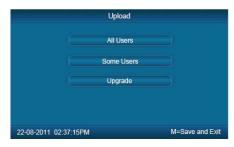
Select 【All user】/ 【Some user】 and press 【OK】 key, will upload the "YG", "ZW" or "NYG", "NZW" two folders to the attendance device. If the two folders not existed in USB pen driver, it can't be uploaded successfully.
