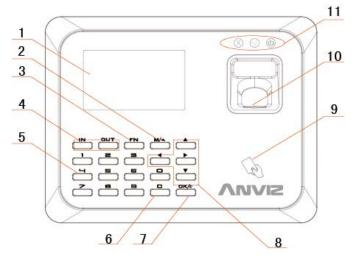
1 LCD LED Indicator 7 Confirm/Power Key
