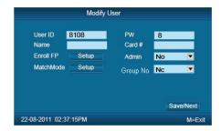
Input the user ID to modify, and press 【OK】 to confirm. The user information will display automatically, and now you can modify user information .Press 【M】 to save .
