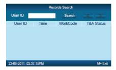
Press 【OK】 and fix cursor to user ID field, input user ID and click 【OK】 to confirm, select 【 ◀ 】、【 ▶ 】 key to move cursor to 【Search】, click 【OK】 to confirm, and all T/A records of this user would be displayed as following.
