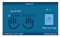
The default fingerprint registering order: 0、1、2、3、4、5、6、7、8、9. Select one finger to register by pressing number keys or 【 ◀】、【▶】 key, then press the same finger 2 times in correct way following the prompt voice.
