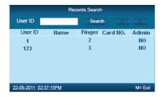
Move the cursor to the user ID field and input user ID, EX. 8248. Press 【C】 to delete when input error and input again, then press 【OK】 to confirm. And press 【Search】 the use information will display in the list.
