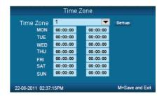
The Time Zone use to setting the time period for access control. The C5 device support 32 time Zones. Setting the time Zone number first and there are two columns setting the time for each day. The first column is the start time and second is the end time.
