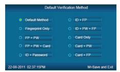
Press 【 ▲】、【 ▼】 key to set the verify method as default method or other personal method. And press 【M】 to save and exit register user.
