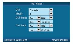
[Modify]: Modify forwards the daylight saving time as N hours.
