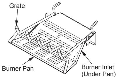
Figure 1 - Product Identification (Ramp Pan Burner)
