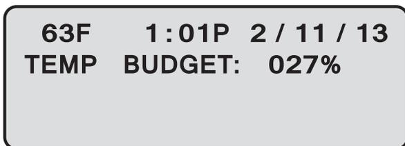
With display shown above, the controller is idle, and awaiting the next start time. Change the time and date on this display as follows:
