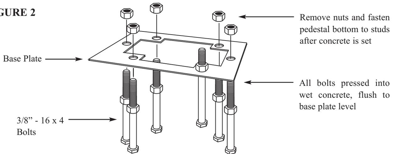
**Step 6)** Prepare fast setting concrete and pour into form, around conduit(s). Immediately trowel and insert base plate with bolts (bolt heads into concrete) and collar around conduit(s). The bracket should "float" on the concrete surface. Verify no tilt by using a level. Allow concrete to set-- typically 1 hour. Troweling should be done in a manner to allow collected water to tread off from pad.
