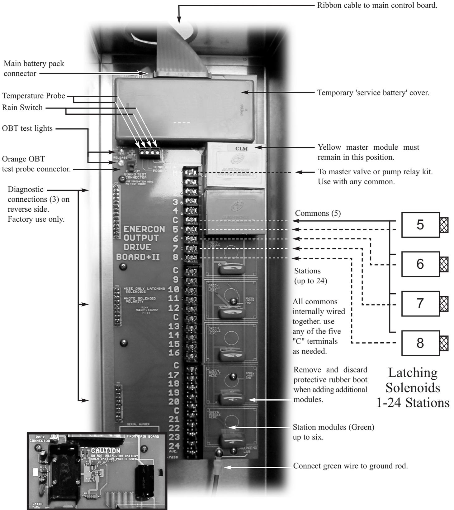
Top of the terminal board showing temporary 9 volt service battery location (cover removed.)
