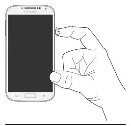
**Note:** Your phone's internal antenna is located along the bottom back of the phone. Do not block the antenna; doing so may affect call quality or cause the phone to operate at a higher power level than necessary.
