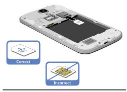
**Note:** If the SIM card is not inserted correctly, the phone cannot make a network connection.
