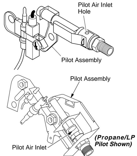
Figure 22 - Pilot Inlet Air Hole
