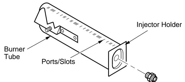
Figure 23 - Injector Holder On Burner Tube
