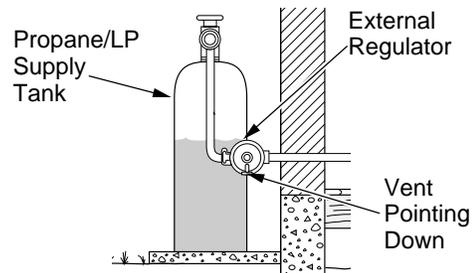
**Figure 12 - External Regulator With Vent Pointing Down**
