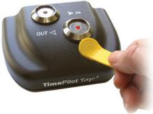
When employees tap their iButtons to the battery-powered Tap<sup>+</sup>, the clock saves three things to its memory: the iButton's serial number (which identifies the employee), the time and date and whether it's a clock-in or a clock-out.
