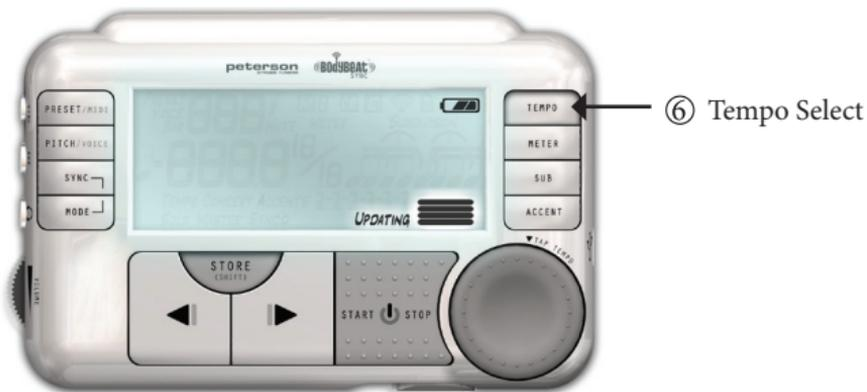
Plugging the BBS-1 into the USB port may automatically turn the unit on in some cases. Holding down the ⑥ Tempo Select Button when this happens will result in the BBS-1 loading into Update Mode as well.
