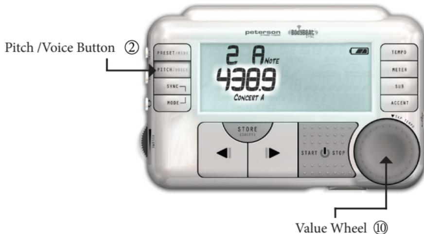
*Note: Pressing the ⑮ Start/Stop button at any time while in Tuning Mode will revert back to Metronome Mode and begin playing the current Metronome settings. Also, pressing any button related to the metronome function will revert to Metronome mode.*
