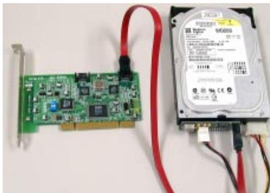
**NOTICE:** The serial ATA cable is used to transfer data of very high frequency. It is suggested not to connect and disconnect it often, for the connector is easily damaged.
