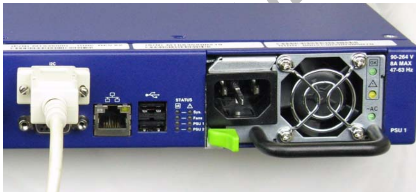
Figure 8: I2C Cable Connected to MTS3600
