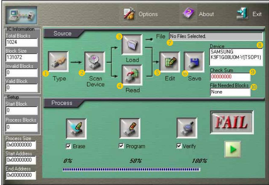
① **Type:** Select IC manufacturer, number and package, also set the Block Size of Code Area (Setting Block Size described in advanced option instruction)
