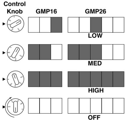
Figure 20 - Burner Patterns for Non-Thermostat Models
