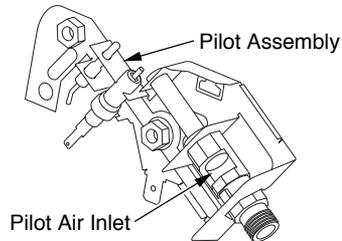
*Figure 30 - Pilot Inlet Air*
