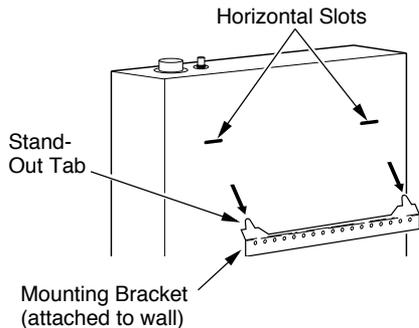
Figure 11 - Mounting Heater Onto Mounting Bracket
