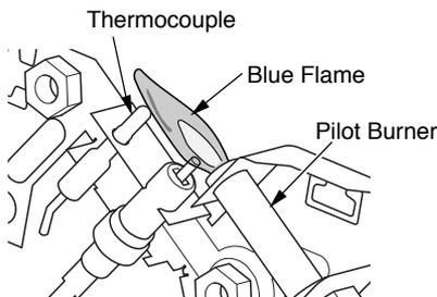
**Figure 24 - Correct Pilot Flame Pattern**
