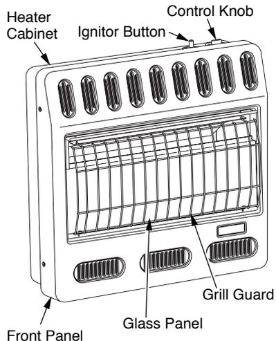
Figure 1 - Vent-Free Gas Heater
