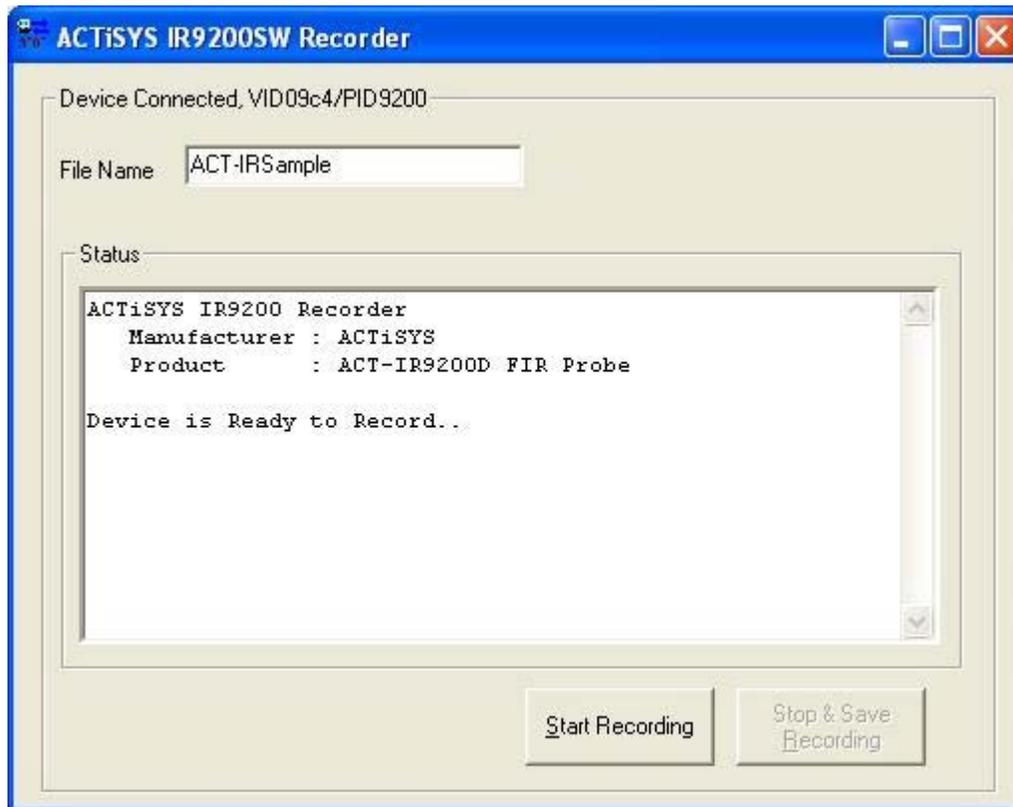
2. Press "Start Recording" button to initiate the Recording. System automatically starts the data collection from the ACT-IR9200D device. After completing the recording, press "Stop & Save Recording" button.
