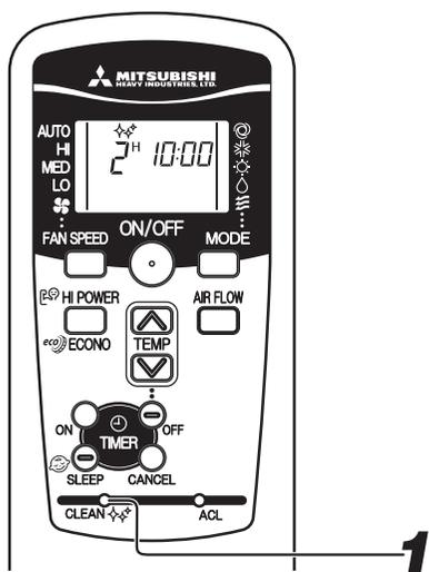
**1** In order to active CLEAN operation, press the CLEAN switch with the tip of a ballpoint pen.
