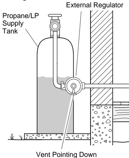
**Figure 14 - External Regulator with Vent Pointing Down**
