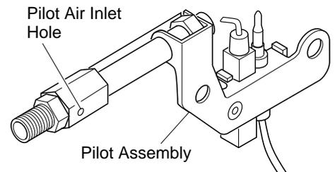
Figure 28 - Pilot Inlet Air Hole
