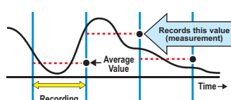
Recording by Average Value Records the average value of the measurements taken every second (or every two seconds) within the set recording interval.
