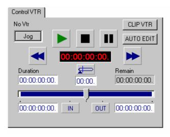
When IN and OUT points are defined, the Auto Edit button starts the playback of the VTR (from the IN point to the OUT point, taking into account the preroll duration) and the record of the XT Series Server at the same time.
