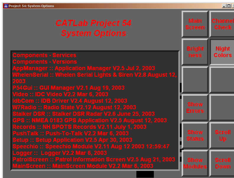
Figure 4. The System Options application with night colors activated. The text field lists currently installed modules.
