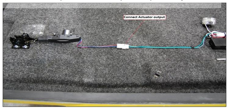
4) Connect Tonneau Harness to the Receiver. If using the optional in cab remote button, connect the gray wire from the Tonneau Harness to the gray wire on the Receiver. Route the Tonneau harness wire up the center of the tonneau cover then over to the driver side front corner of the box. Mount the harness with supplied Cable Clamps and screws or under the carpeted head liner. Leave the end of the harness accessible to be able to later connect it to the Truck Harness.
