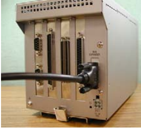
Figure 2.9. Connecting the connection cable to this product
