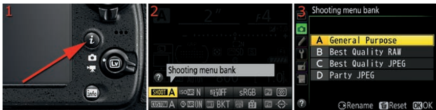
Figure 3.1B – Accessing the Shooting menu banks with the i button and Quick Menu screen
