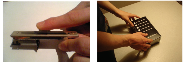
Figure 1. Motorized slider (left) and mock-up box of multi-slider interactive device (right).
