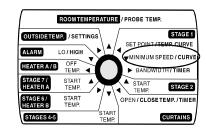
Press the push-button. The word OFF is displayed, indicating that the minimum speed curve is deactivated. If this is not the case, deactivate the curve as described below.
