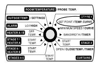
Press the push-button. The word **OFF** is displayed indicating that the termperature curve is deactivated. If this is not the case, see below to deactivate the curve.
