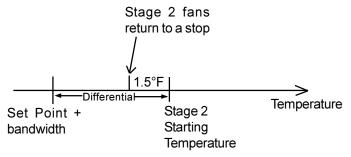
The differential shown above can go from  $0^{\circ}F$  to  $20.0^{\circ}F$  ( $0^{\circ}C$  to  $11.1^{\circ}C$ ). If this value is less than  $1.5^{\circ}F$ , the hysteresis is adjusted to the new differential. If the differential is less than  $0.3^{\circ}F$ , the hysteresis is set to  $0.3^{\circ}F$ . Note that if an SB2000 air inlet controller is being used, the differential must be greater than  $0.5^{\circ}F$  in order for Stage 2 to be interpreted correctly.
