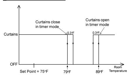
In the example above, when the temperature rises to  $89^{\circ}F$ , the curtains begin to open and continue to do so until fully open if the temperature remains above this point. If the temperature falls to  $88.7^{\circ}F$ , the curtains stop opening.
