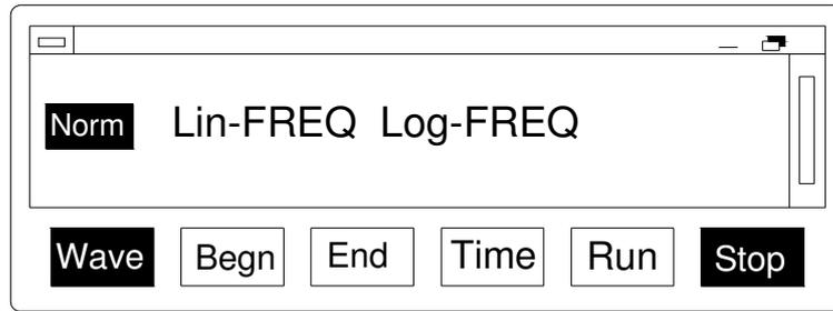
Select output waveforms by direction keys. Functions correspondently to screen menu setting:
