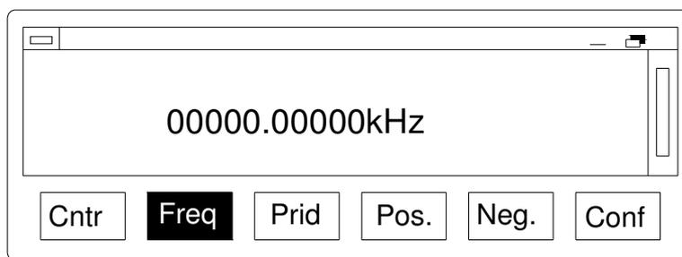
2. press F2 corresponding to frequency to realize frequency measurement.
