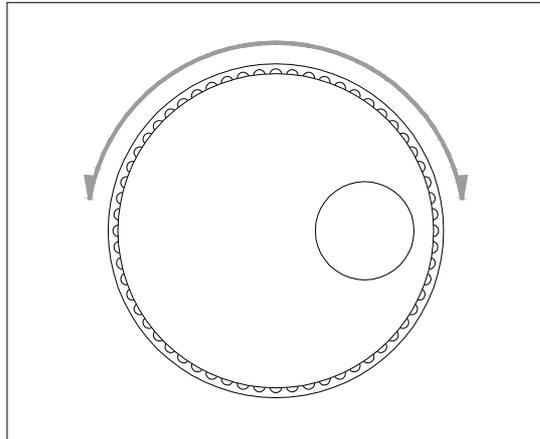
By using rotary pulse switch, you can quickly add or subtract the value which cursor points to, Inputting numbers by this way, it will be more convenient.
