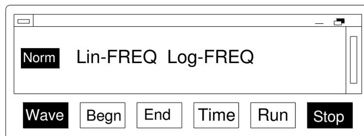
3. press F2 pointing to starting point menu ,set up starting frequency 100kHz
