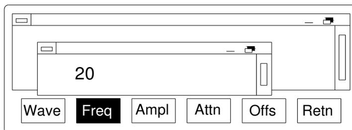
After desired digits had been input, press OK key to confirm the present unit, you also can press amplitude modulation frequency modulation. Press amplitude key to choose Hz, kHz or MHz unit for frequency value. By finishing frequency input, the result is as follows:
