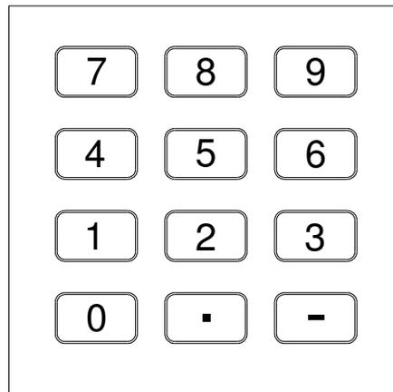
The digital keyboard which is composed of 12 keys, 0-9 digital keys and (.),(-), is designed for fast inputting numbers. When in digital mode, if you press any digital key, a dialogue block will appear on the screen which stores the pressed keys. Then press OK key to confirm.
