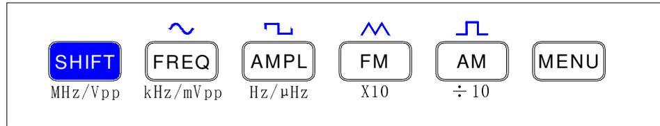
These short-cut keys enable you to implement desirable function quickly and they are keys in common use. Their functions are divided into the following two kinds:
