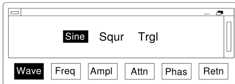
Selecting waveform by direction keys, selecting other parameters of output wave put waveform by F1-F6 (sine wave, square wave, triangle wave)
