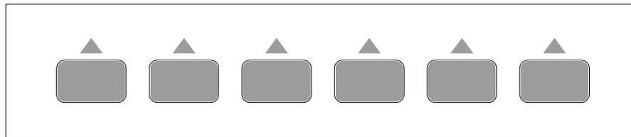
Screen keys are special function keys set for special screen display. From left to right ,they are respectively called F1、 F2、 F3、 F4、 F5、 F6. Just as what you think, they are fictitious keys corresponding to the screen one by one .Ex. Channel 1 setting is corresponding to screen wave form ,frequency, amplitude ,bias and return.
