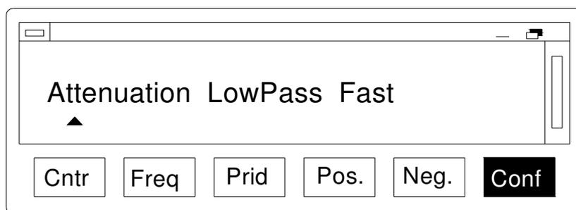
The group state includes: “attenuation”, “low pass filter”, “fast” functions. Return white by direction key left right to select, then press Ok key to change the state.
