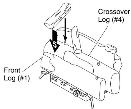
Figure 32 - Installing Crossover Log (#5)
