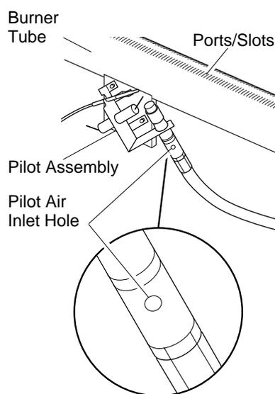
**Figure 45 - Pilot Inlet Air Hole**
