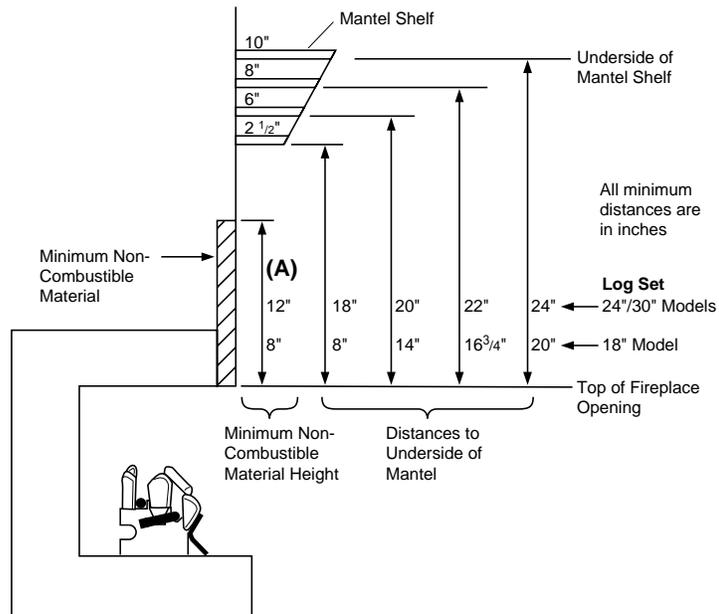
**Figure 7 - Minimum Mantel Clearances Without Using Hood**
