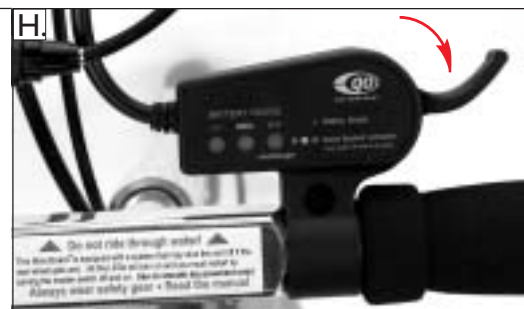
To Accelerate gently squeeze the Speed Controller.
