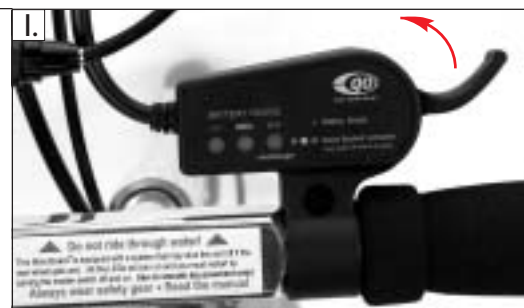
To Decelerate let go of the Speed Controller.
