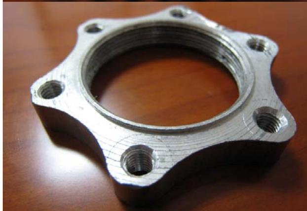
Twist the Disc Brake Plate into position.
