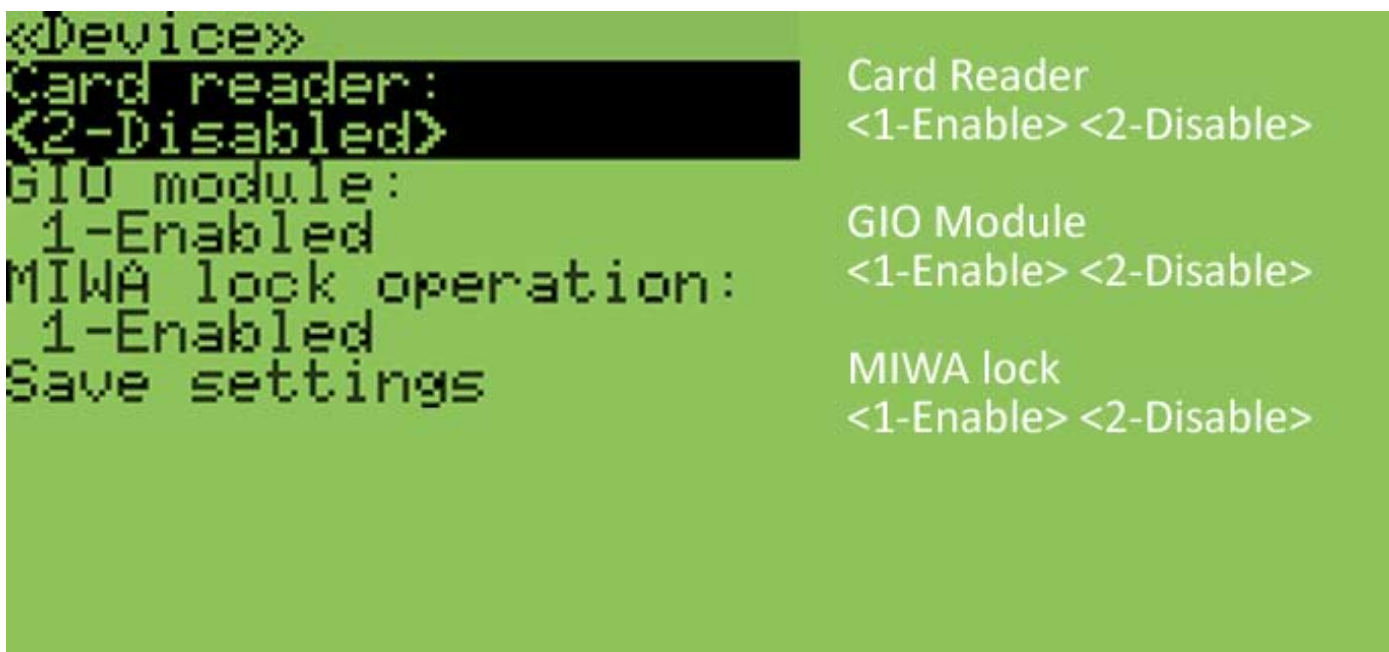
Fig. 47 - In “Device” section, is possible to enable/disable proximity card readers, GIO Module and a MIWA lock
