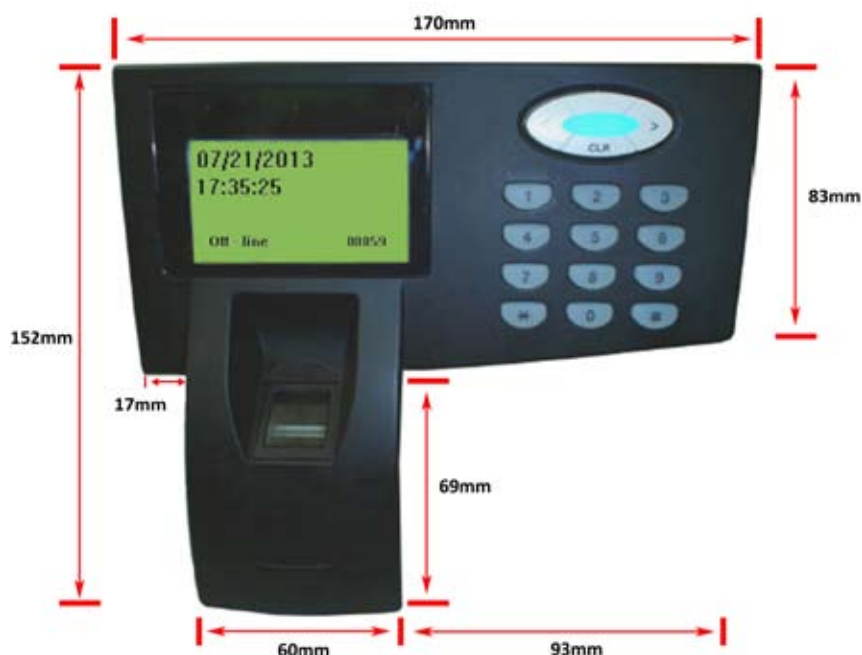
Fig.3 - GAM 110 unit dimensions - FRONT
