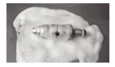
4. Clean with detergent. Clean the device manually under running warm water using an enzymatic cleaner or detergent for a minimum of 5 minutes. Manipulate all moving parts under running water. Use a soft-bristled brush and/or soft lint-free cloth to remove all visible soil and debris
