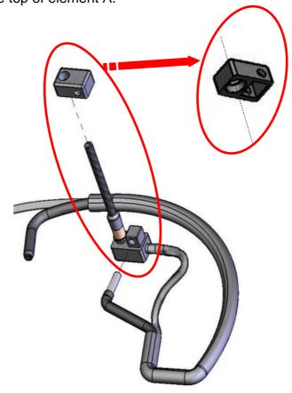
**Step four**: connect the ending of the over-ear microphone to the side hole of element A.
