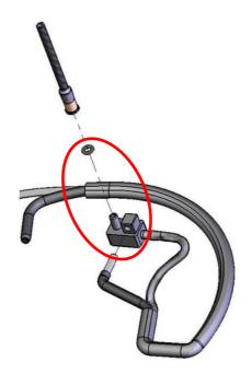
**Step three:** mount the microphone housing (A) on the probe putting the probe through the hole on the top of element A.
