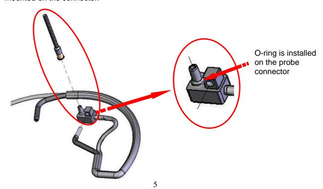
Use the spare o-ring only in case the original one is not placed on the connector:
