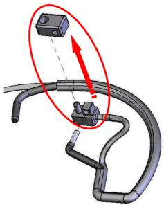
**Step two:** place the microphone probe (D/F) on the connector making sure that <u>one</u> o-ring (B) is placed between probe and connector. In a new set the o-ring is already mounted on the connector.
