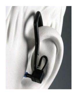
Take caution whenever the microphone is placed inside the human ear. Correct position for probe placement is the entry of the ear channel **not inside of it!**Otherwise sudden movements of the user or unexpected blows around ear area may cause serious injuries if enough carefulness is not kept.
