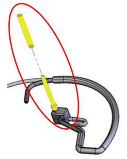
Before placing the SV 25S microphone in the ear remember to put the silica pipe on the probe.
