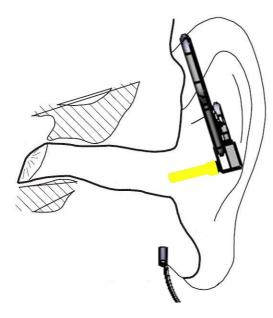
SV 25S microphone measures sound pressure level in the ear canal by means of the probe which is placed at the entry to the ear canal. The length of the probe is 16mm to ensure the maximum comfort and protect from contact with the eardrum.
