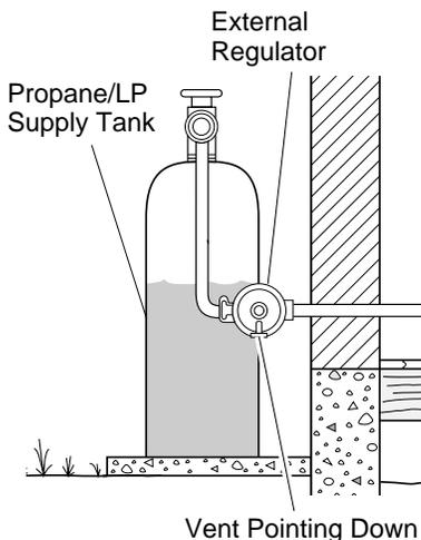
Figure 20 - External Regulator with Vent Pointing Down
