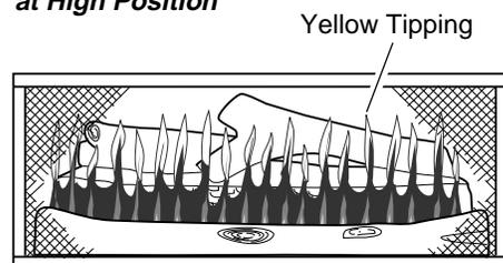
Figure 29 - Incorrect Burner Flame Pattern at High Position
