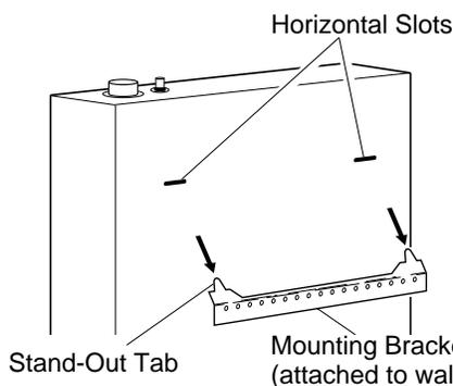
Figure 16 - Mounting Heater Onto Mounting Bracket
