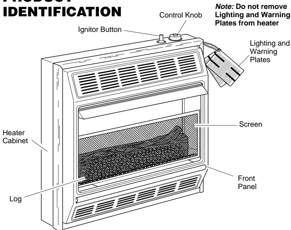
Figure 1 - Vent-Free Gas Log Propane/LP Gas Space Heater
