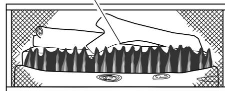
Figure 28 - Correct Burner Flame Pattern at High Position
