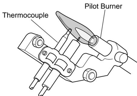
Figure 26 - Correct Pilot Flame Pattern
