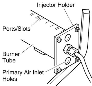
**Figure 30 - Injector Holder On Outlet Burner Tube**
