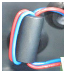
Figure 3-2: Ferrite core and battery supply wiring
