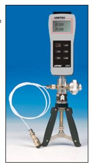
A special quick connector between the pump and the indicator makes it possible to seperate the system in seconds.
