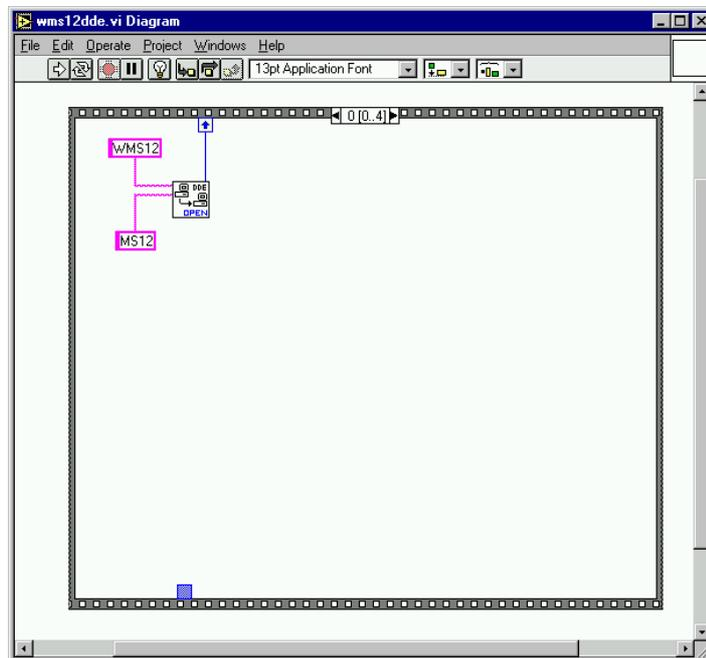
Figure 4.8: Opening the DDE conversation with the WMS12.EXE in LabVIEW
