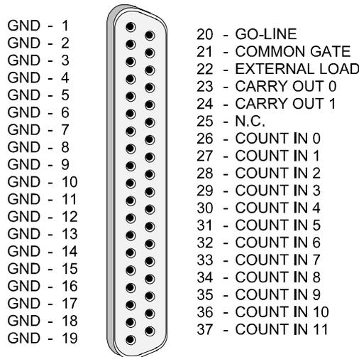
**Figure 3.3: Connector Assignment D-SUB 37**
