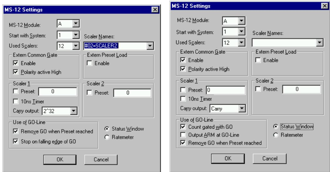
**Figure 4.2: MS-12 Settings dialog, left: used with MCD4LAP, right: with MPA-3**
