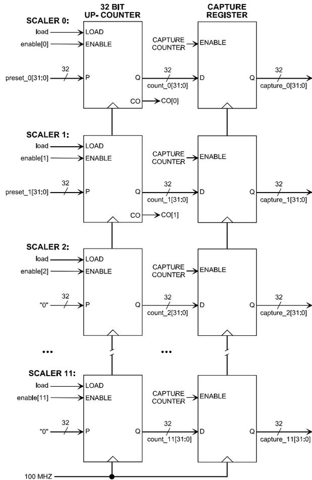
Figure 3.1: Simplified Block Diagram of Counters
