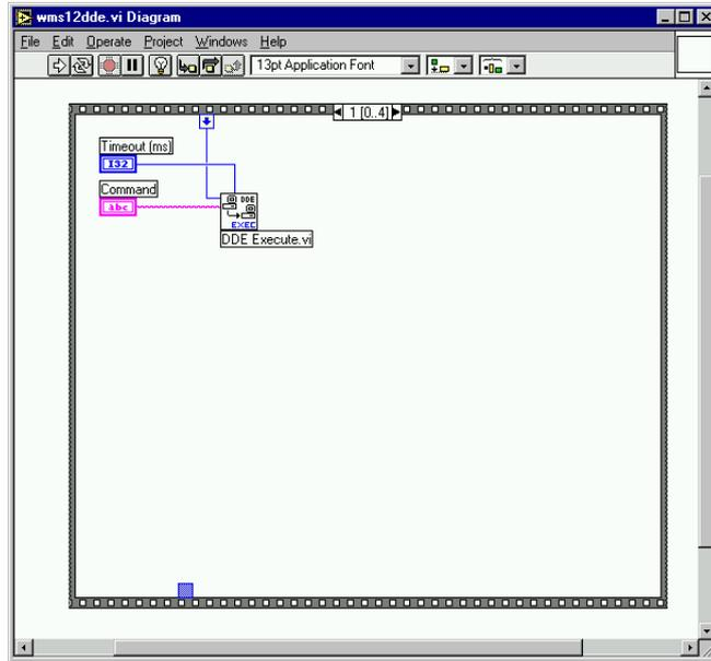
Figure 4.9: Executing a WMS12 command from a LabVIEW application
