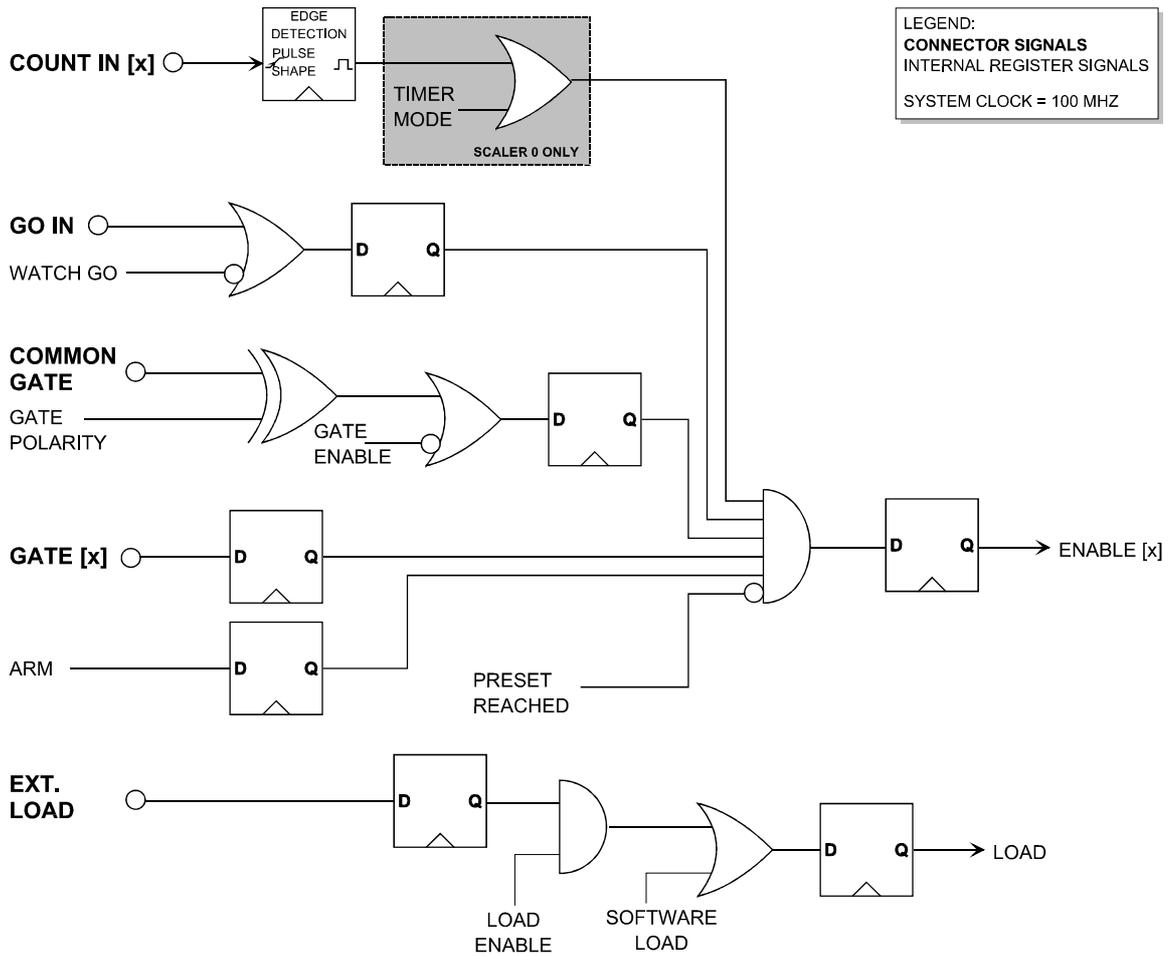
Figure 3.2: Schematic of Scaler Inputs
