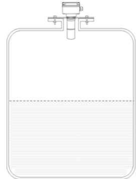
lengthen sensor to shun frost and icing
