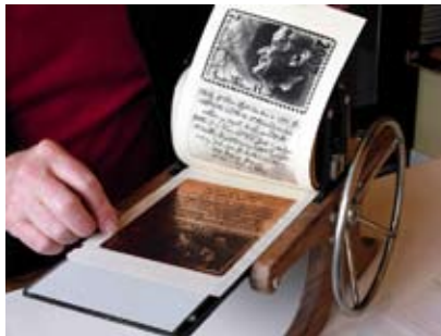
Examine it for tone, clean, full lines that show uniform, adequate pressure.
