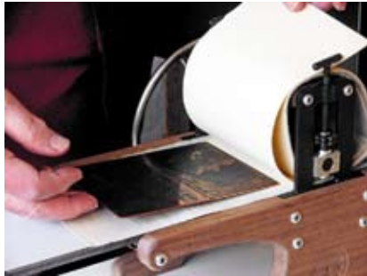
Put a piece of damp newsprint under the plate first, then put the plate on this damp paper so it will not slide.
