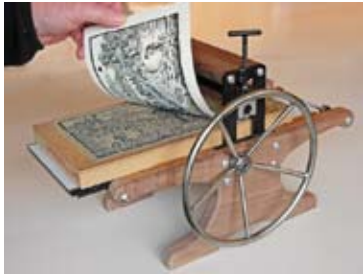
Type-high means that the printing block is the same as moveable type from traditional letterpress printing. Mounted linoleum is sold by companies such as Speedball. The illustration shows a block the same size as the press bed.
