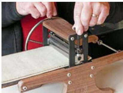
Turn the pressure screws clock-wise to tighten. The illustration shows the felt blankets are under the roller when you set the pressure, and use two hands so the chain is not stressed.
