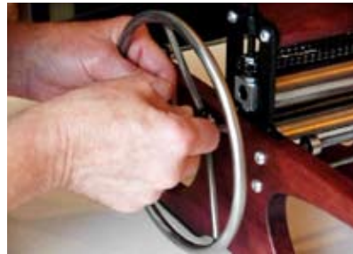
The illustration shows the larger hex key in the set screw on the driving wheel. The set screw is aligned with a flat place on the shaft.
