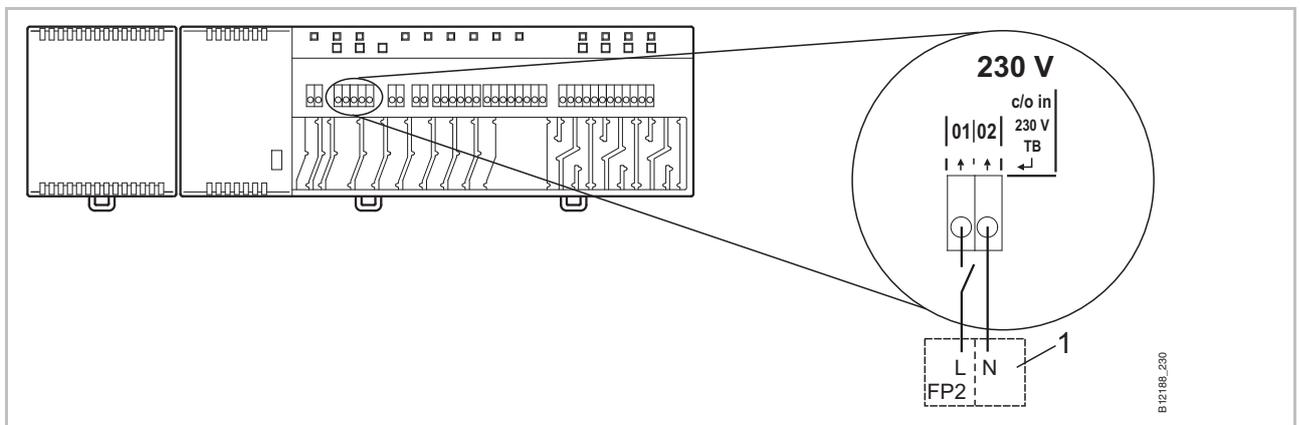
Fig. 24: TB-input, control with 230 V
