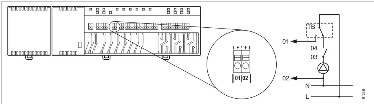
Fig. 25: TB-input for temperature monitoring
