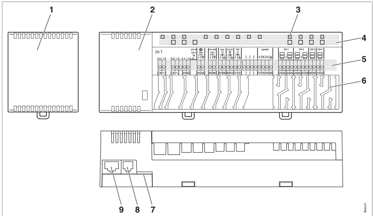
Fig. 2: Design wireless connection module, 4-channel version shown.
