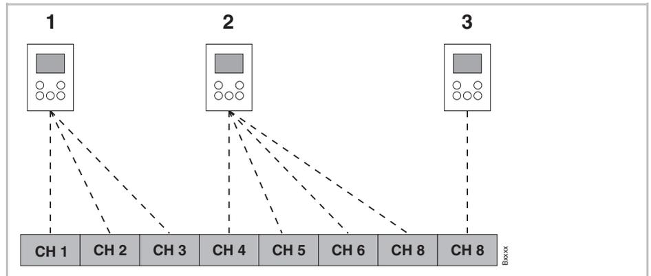
Fig. 42: Radio channel group with equal priority
