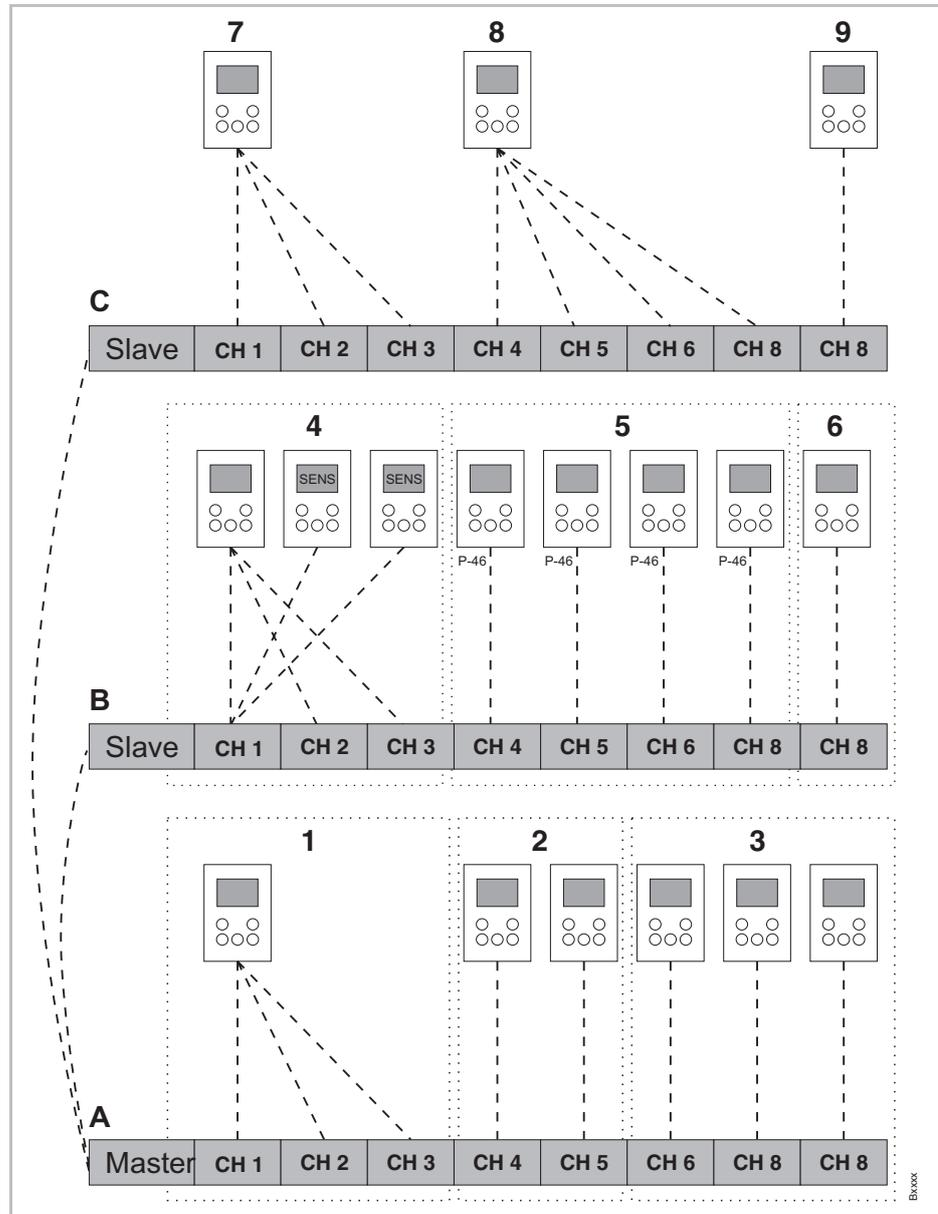
Fig. 48: Example with three wireless connection modules
