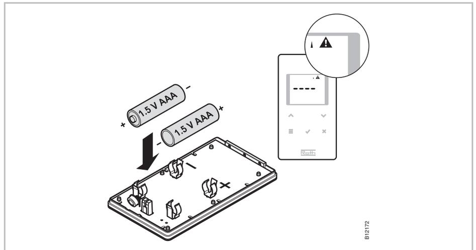
Fig. 12: Insert batteries
