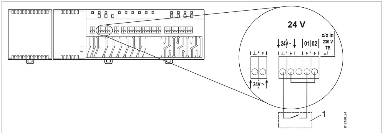
Fig. 23: TB-input, control with 24 V voltage from wireless connection module
