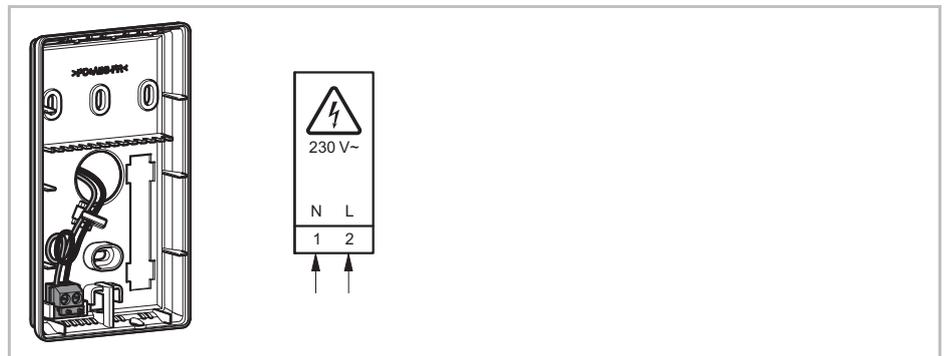
Fig. 15: Close the wireless room thermostat
