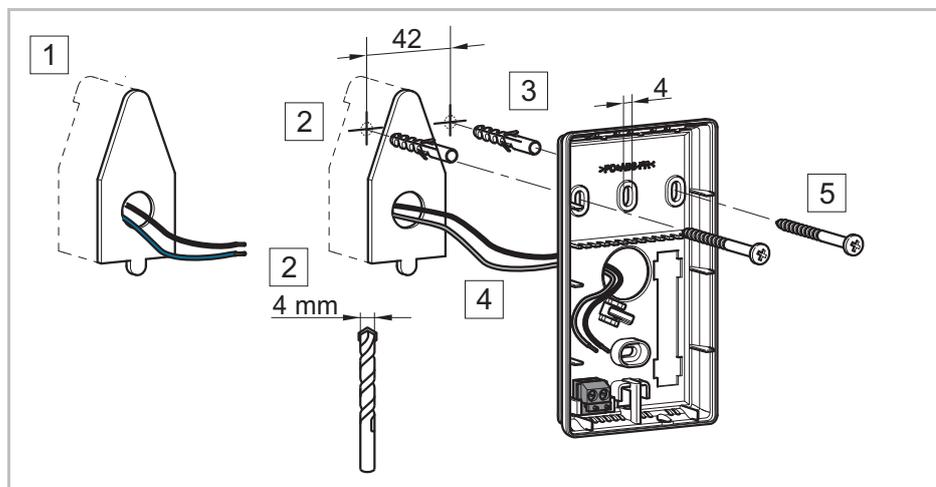
Fig. 14: Installation bottom part of wireless room thermostat
