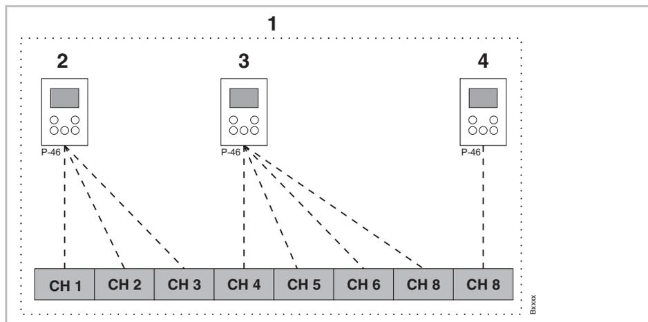
Fig. 45: Setpoint sharing for all wireless room thermostat within one zone
