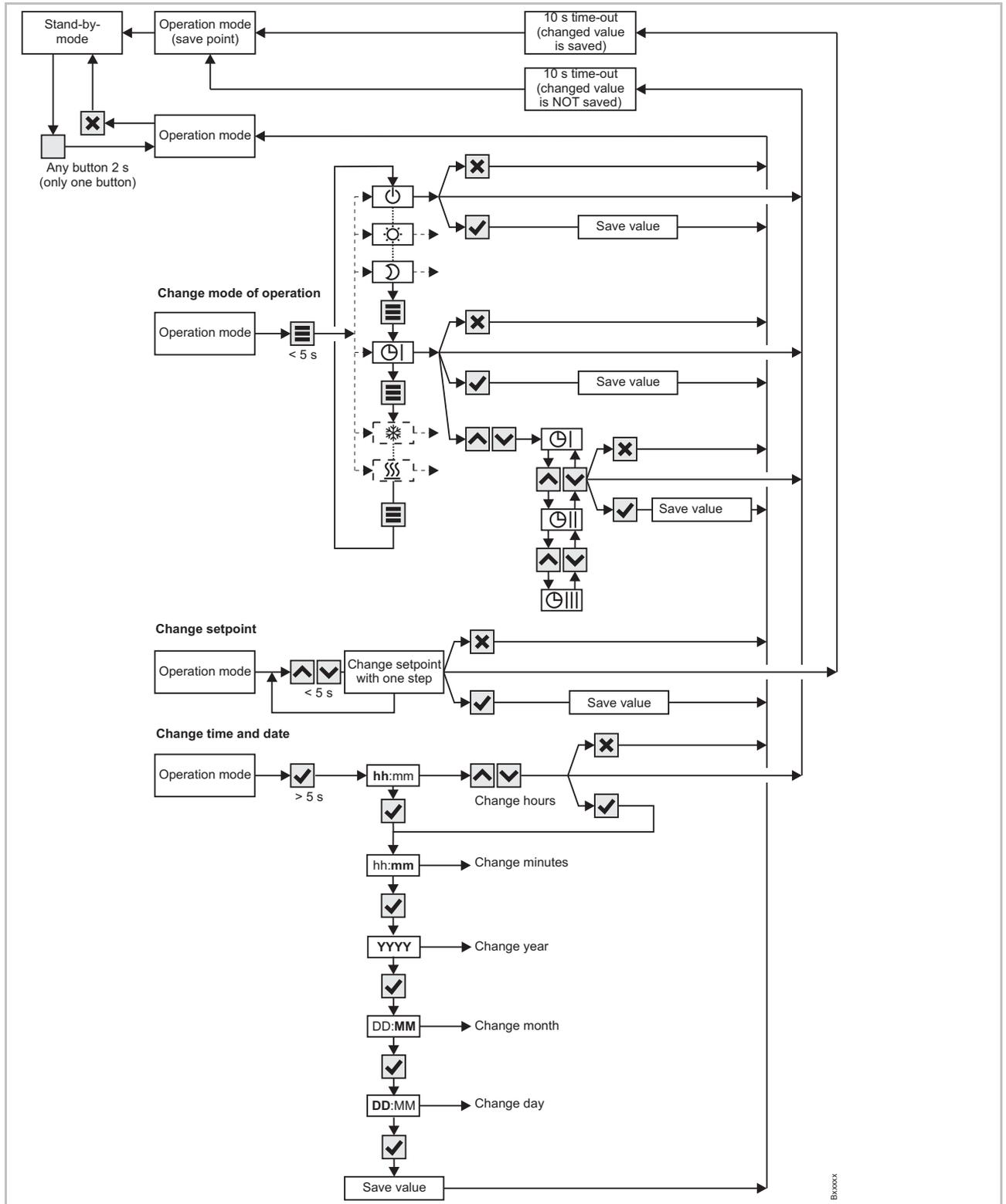
Fig. 40: Menu structure operation
