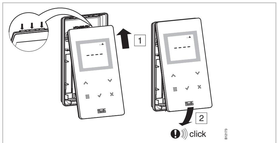
Fig. 13: Close the wireless room thermostat
