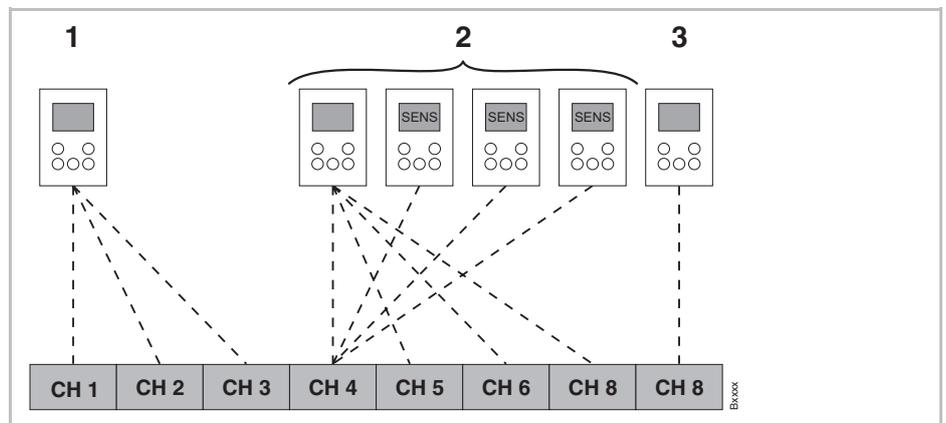
Fig. 43: Radio channel groups with equal priority and average temperature building
