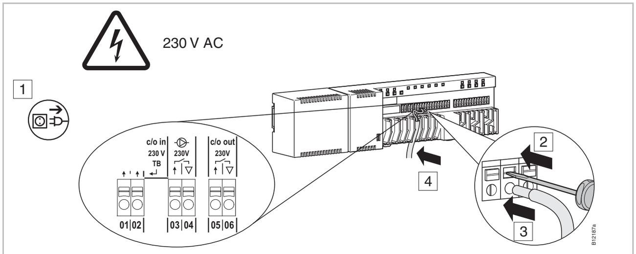
Fig. 19: Connect wires
