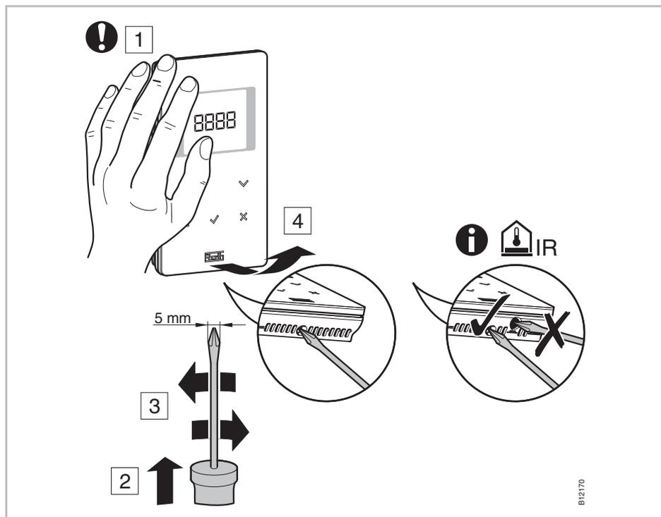
Fig. 10: Open the wireless room thermostat
