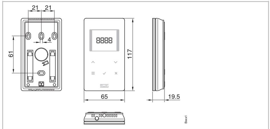
Fig. 39: Dimensions wireless room thermostat
