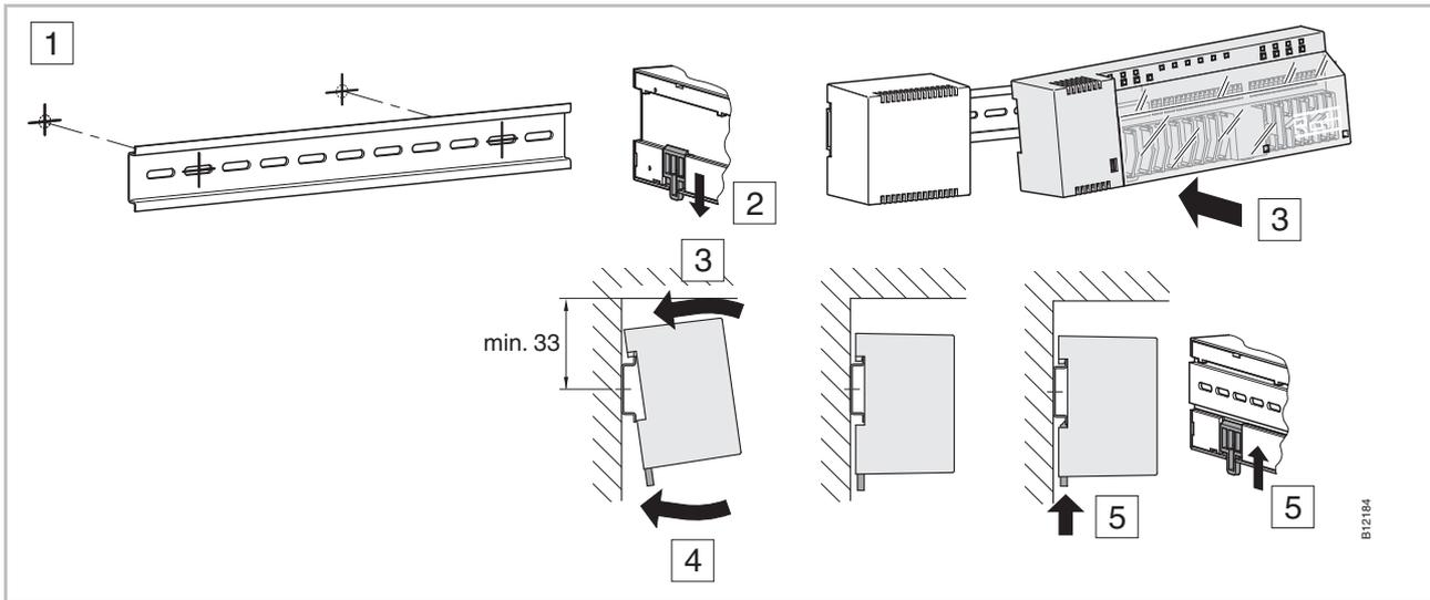
Fig. 7: Installation wireless connection module
