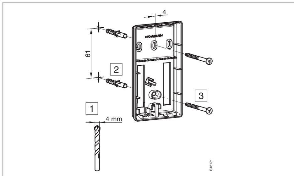
Fig. 11: Installation bottom part of wireless room thermostat
