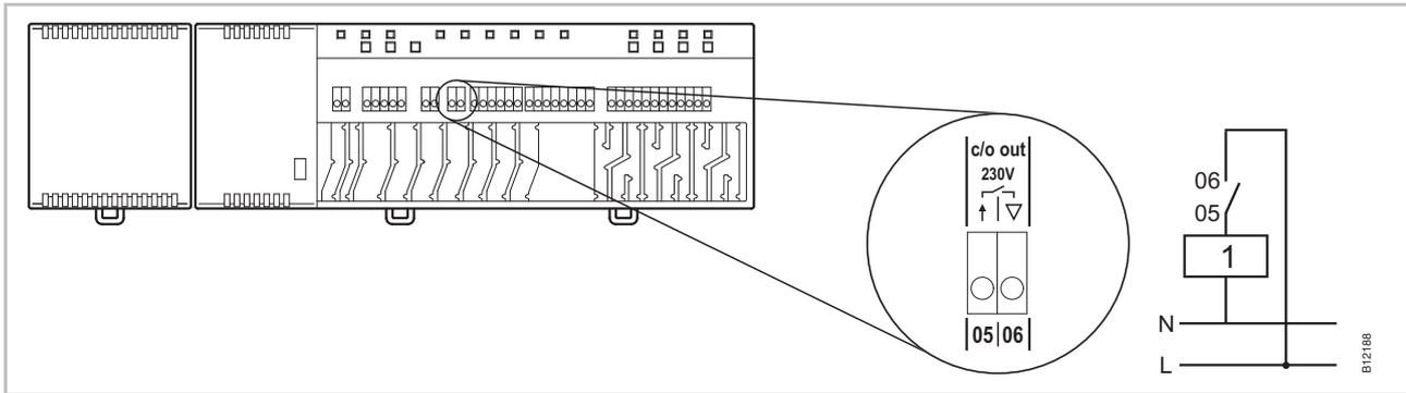
Fig. 21: C/O- or burner output, 230 V
