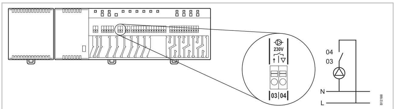
Fig. 20: Connect pump, 230 V
