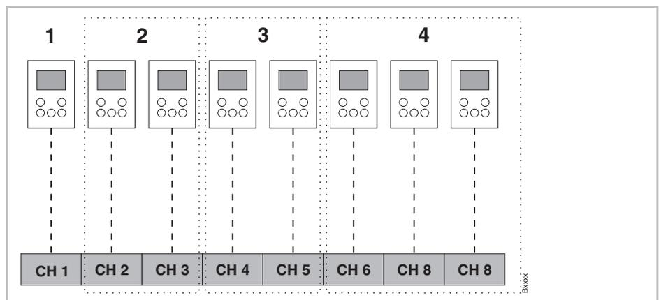
Fig. 47: Wireless room thermostat as "Master" for mode of operation
