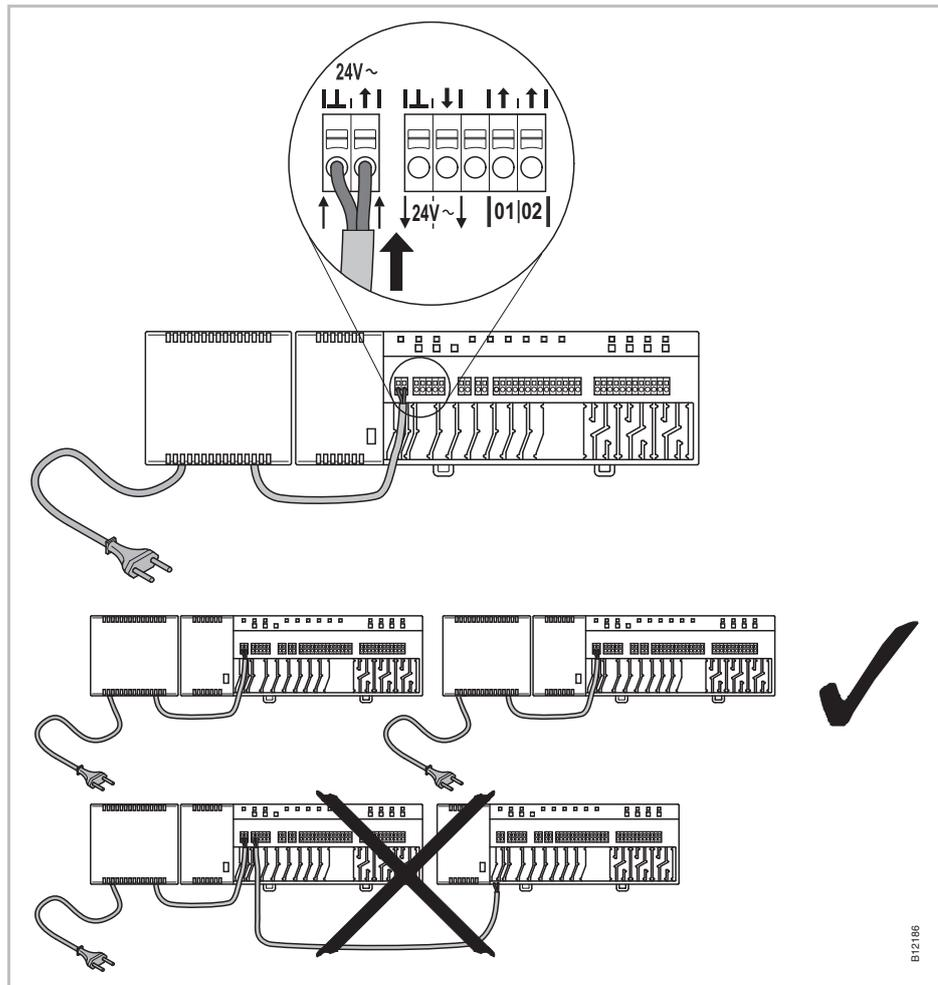
Abb. 18: Connect transformer
