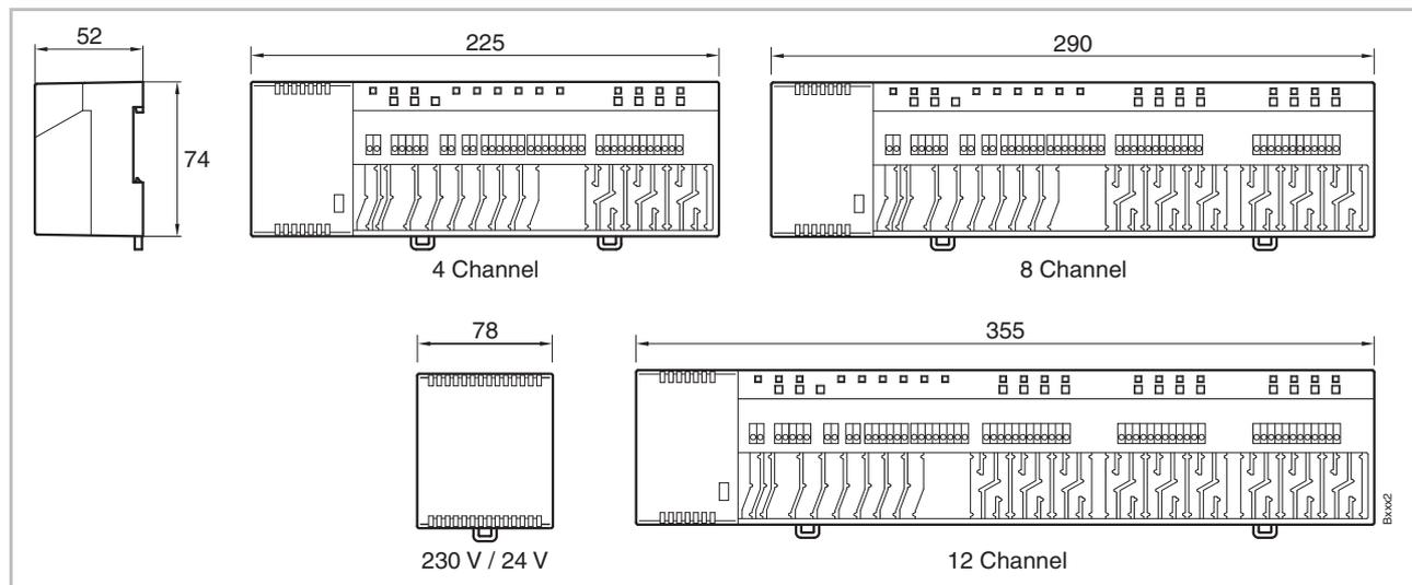
Fig. 38: Dimensions wireless connection module with transformer
