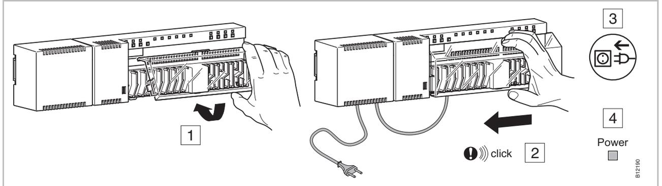
Fig. 30: Install cover and connect power supply
