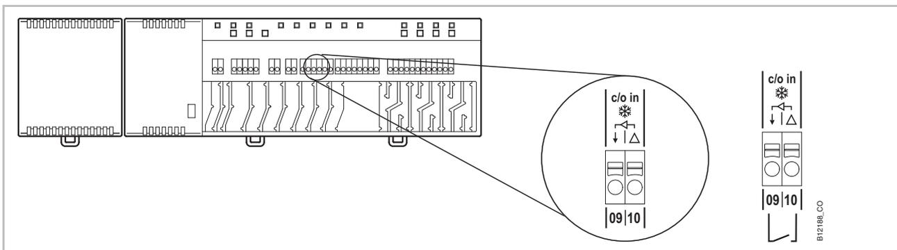
Fig. 26: C/O-input, potential free contact
