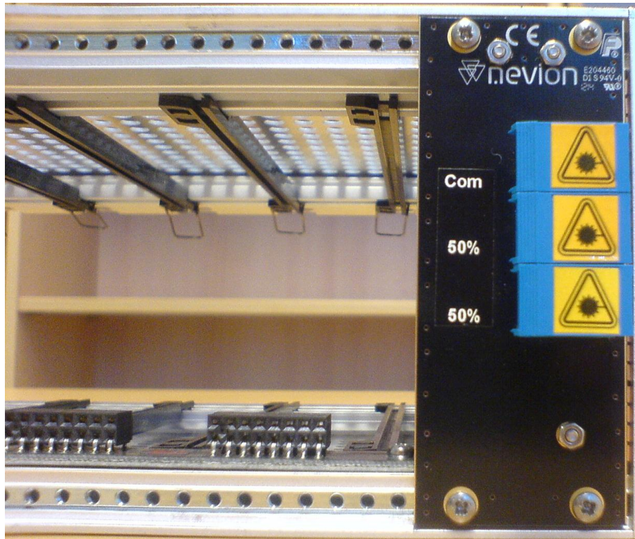
Figure 8 WOC-2-50-50 Mounted in a Flashlink sub rack
