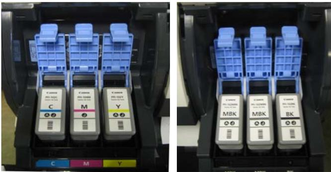
The imagePROGRAF iPF750 utilizes 5 color inks. The three colored (C, M, and Y) ink tanks are housed on the top left side of the printer, and three black (B and MBKx2) ink tanks are located on the top right side.
