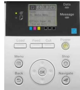
After installing new media, the LCD panel on the iPF750 prompts the user to specify the newly installed paper type. You should note that the iPF750 printer automatically detects media width.
