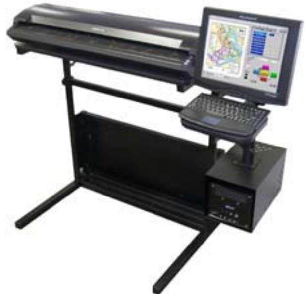
*The Graphtec SK280 is only sold bundled with the EIS MFP solutions and not sold by itself. The Graphtec SK280 scanner uses five A4 sensors in a zigzag pattern.*
