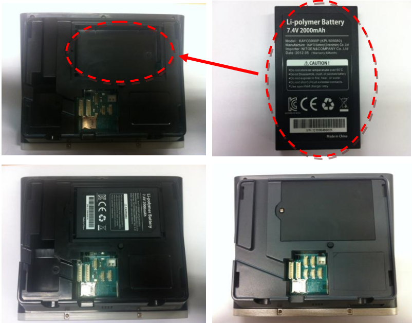
Figure 3.2 Installation of battery
