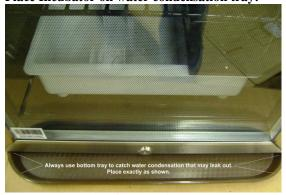
Choose the location for operation & place the condensation tray under the front portion of the incubator as shown.
