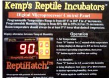
Firmly press the "S" button for ½ second while the humidity is being displayed (not while temperature is being displayed). Then adjust the desired incubation humidity by pressing the UP and DOWN button on the display. After selecting the humidity firmly press the "S" again. The alternating display will change to show the current temperature & humidity conditions inside the incubator. The settings will also be maintained during a power failure.
