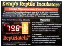
Firmly press the "S" button for ½ second while the temperature is being displayed (not while humidity is being displayed). Then adjust the desired incubation temperature by pressing the UP and DOWN button on the display. After selecting the temperature firmly press the "S" again. The alternating display will change to show the current temperature & humidity conditions inside the incubator. The settings will also be maintained during a power failure.
