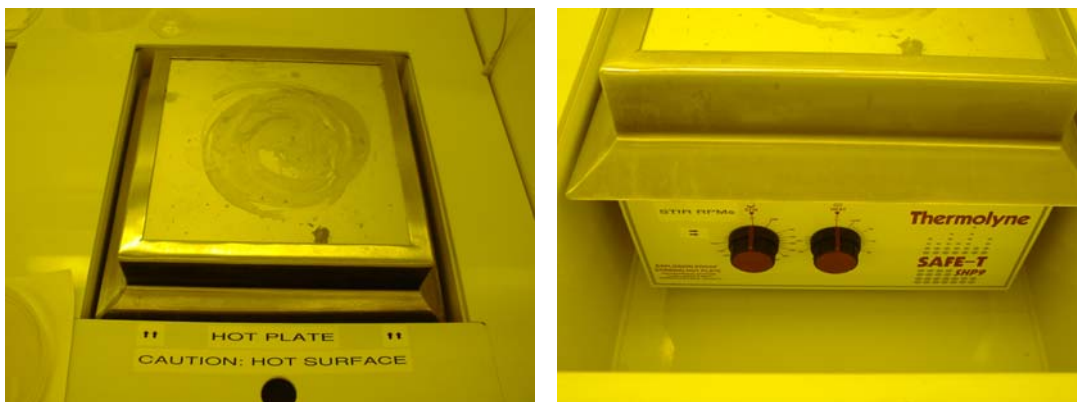
Figure 5. Stirring, explosion proof manual hotplate showing protective skirt and controls under the removable panel.
