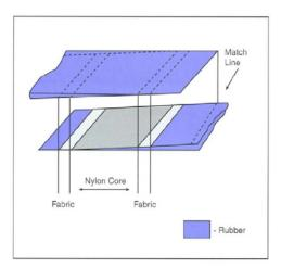
Joint Belts Without Rubber Covers: Types SG, TAIR, TTA, and KSG belts use only Polybond A solution. Do not use excessive amounts of solutions. Too much causes a weak bond.
