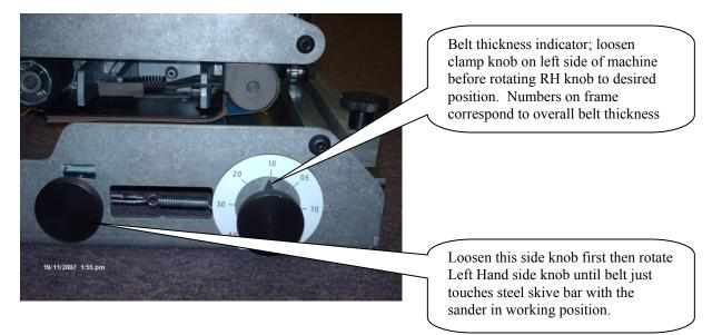
For best results, always make sure the steel skive edge bar has a square corner. If corner is worn, rotate skive bar to fresh edge, or replace as required.
