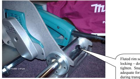
Fluted rim screw for locking – do not over tighten. Snug tight is adequate for holding unit during transportation.
