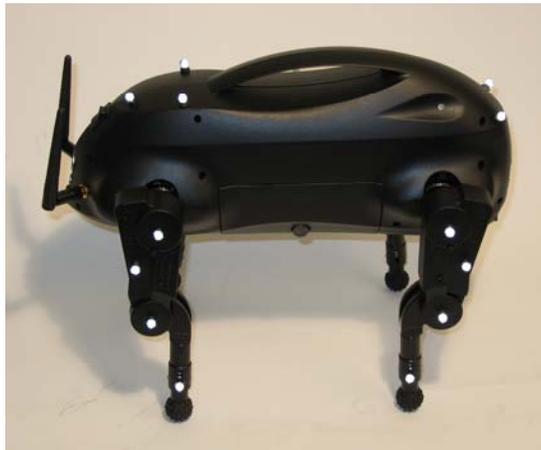
**Figure 6: Robot Zero Configuration Position**
