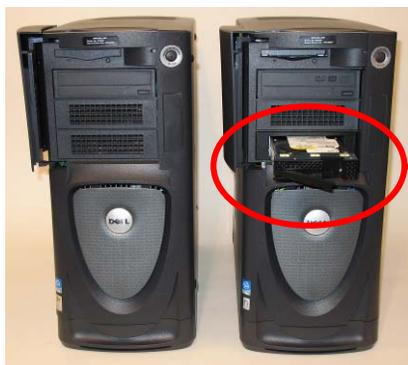
The HOST computer can be identified by the removable hard drive accessible in the drive bay. Additionally the MoCap PC is marked with a Windows XP sticker near the bottom left of the case.
