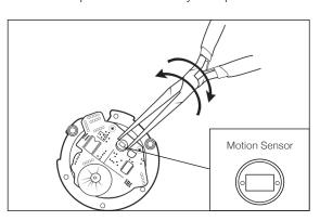
3. Pull the face apart from the battery compartment. Locate the motion sensor (a circle with a black rectangle inside). The motion sensor can be removed with needle nose pliers, gently twisting until it detaches from unit.
