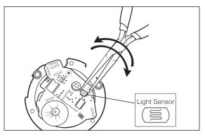
4. Remove light sensor with needle nose pliers, gently twisting until it detaches. Replace battery compartment into face of the light. Screw six screws securely and twist back to base of light. See your user manual for installation instructions.
