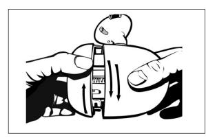
1. Remove front cover of Spotlight by rotating counter-clockwise as shown above. Pull face out from cup to reveal battery compartment.
