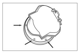
2. Remove the six screws on the inside of the face of the Spotlight.
