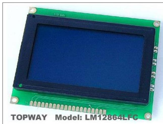
*Figure 2: LM12864LFC LCD*
