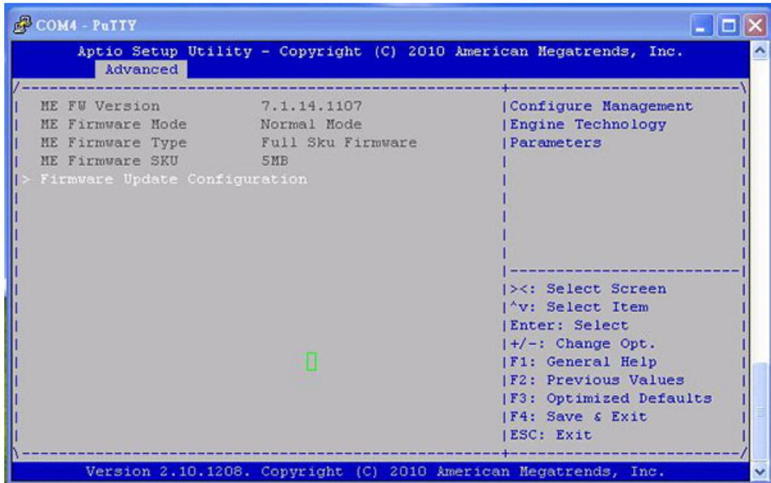
Figure 4.12 Intel Management Engine firmware configuration menu
