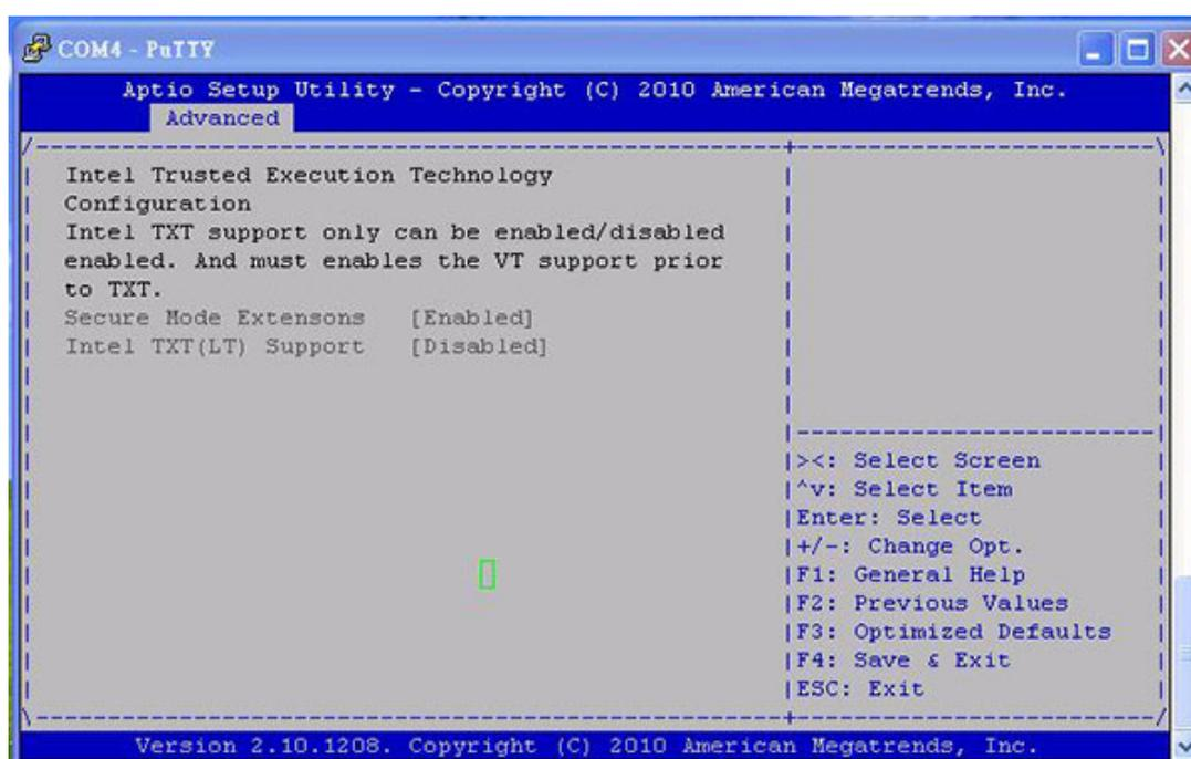
Figure 4.11 Intel Trusted Execution Technology configuration menu
