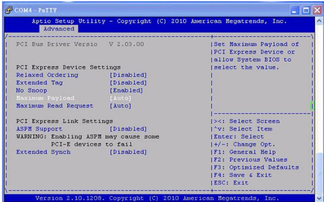
Figure 4.6 PCI Express subsystem settings
