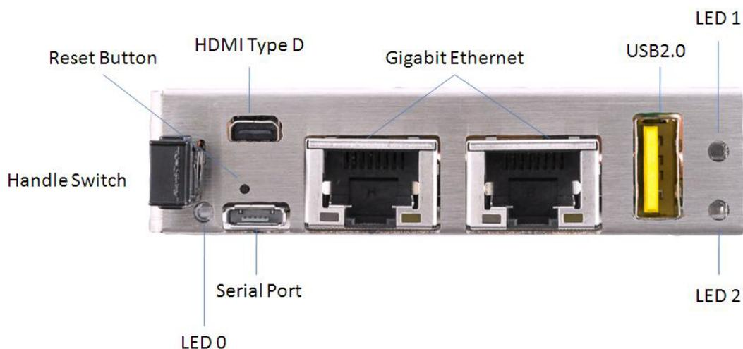
Figure 2.2 MIC-5603 Front Panel
