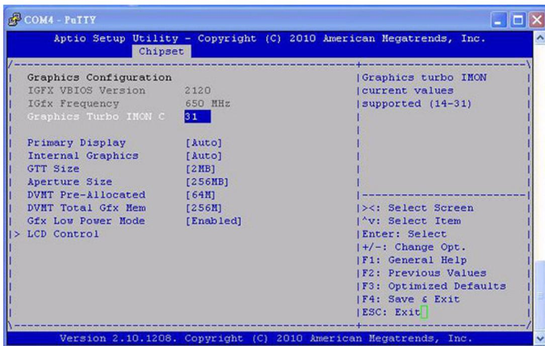
Figure 4.18 Intel graphics engine configuration menu
