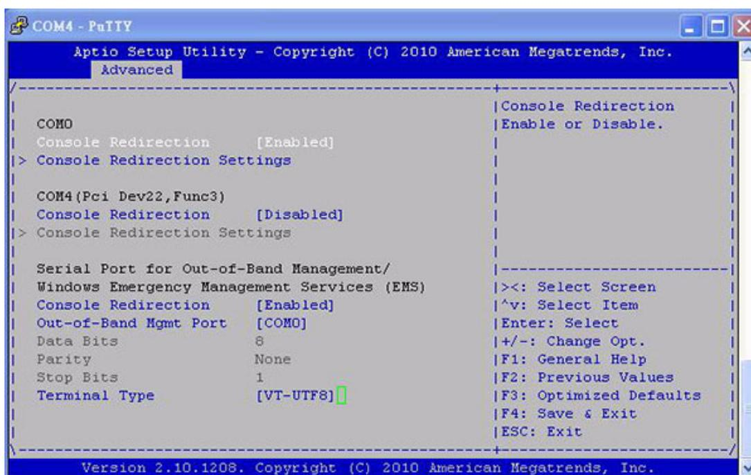
Figure 4.14 Console redirection configuration menu
