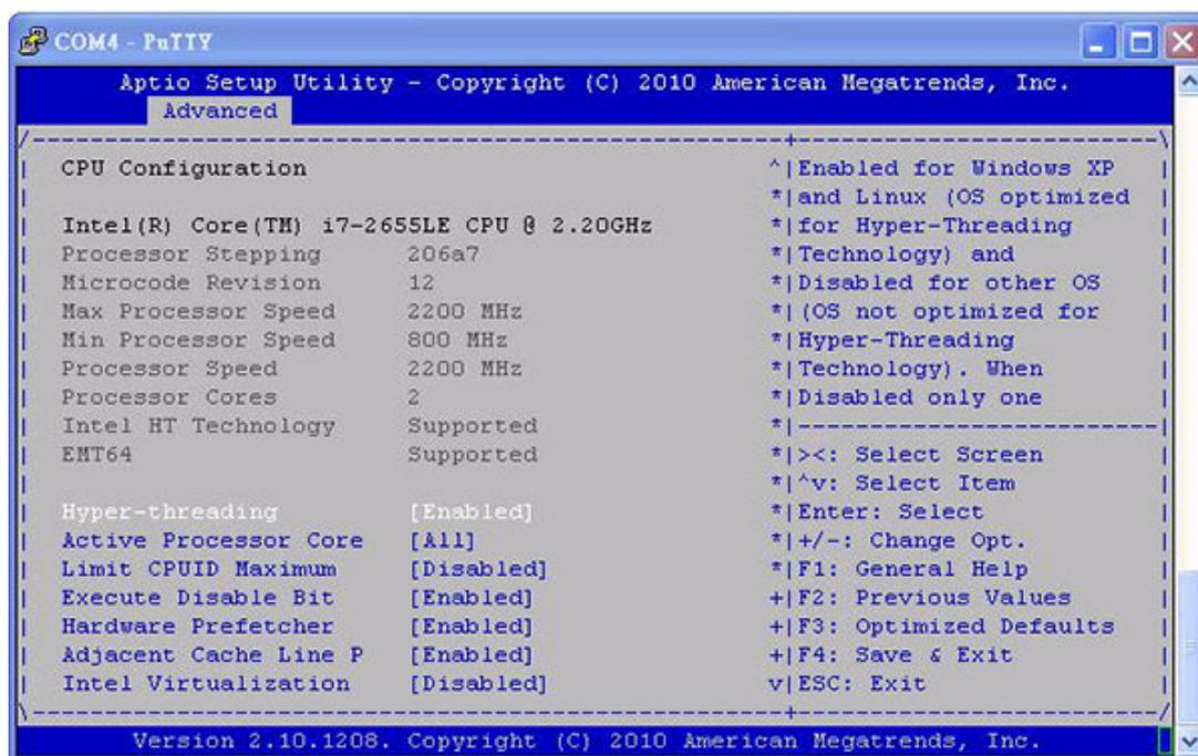
Figure 4.9 CPU Configuration
