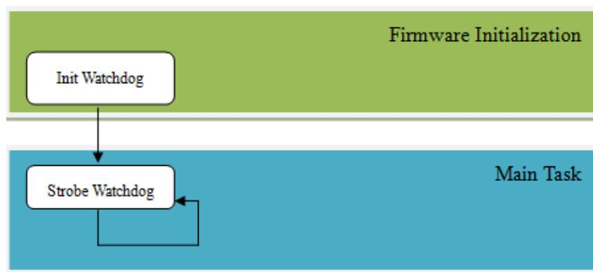
If the Watchdog is triggered, the IPMB-L is isolated from the controller. The AMC Payload is not affected and the FRUs operational state stays untouched.
