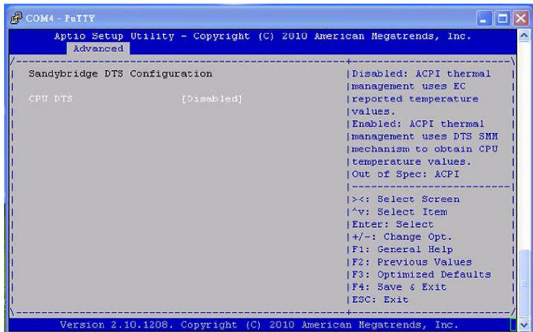
Figure 4.15 Processor Digital Thermal Sensor setting
