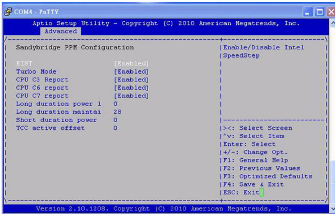
Figure 4.16 Processor PPM configuration menu
