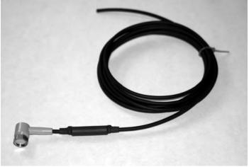
To meet the stated performance criteria, the armor-jacketed accelerometer cable has one (1) ferrite installed. It is a Steward ferrite (part number 28B0672-000), which provides 245 ohms of reactance at 100 MHz.
