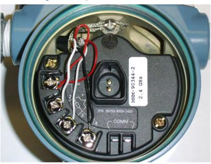
Figure 3-8: Connecting two sensors/accelerometers
