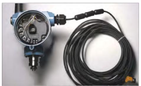
Figure D-8: Ferrites installed on a standard cable
