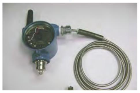
Figure D-9: Ferrites installed on an armor-jacketed cable
