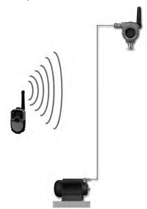
Figure D-12: RFI source polarization coincident with long cable run (maximum interference)
