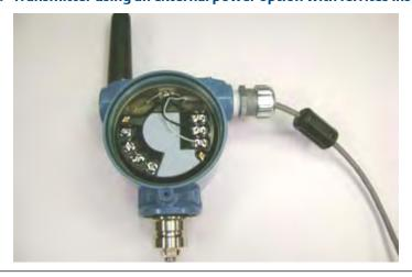
Figure D-10: Transmitter using an external power option with ferrites installed
