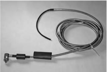
Figure D-5: 3-meter armor-jacketed accelerometer cables with ferrite installed (as
