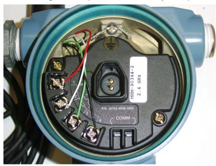
Figure 3-9: Connecting one sensor (accelerometer with temperature)
